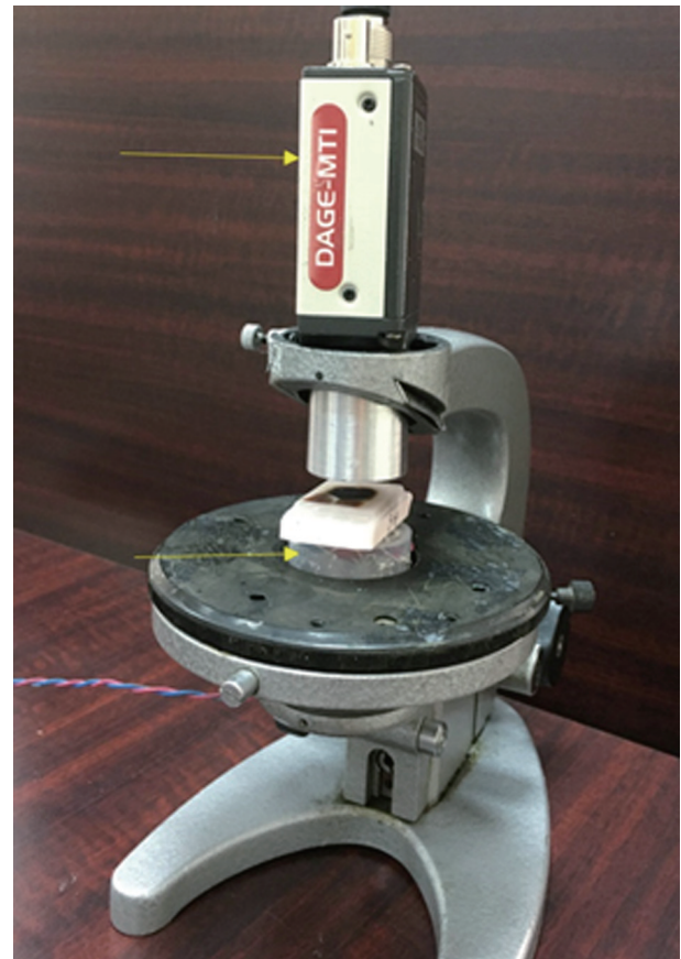
Figure 1. Setup of the experiment. Arrows are used to show the CCD camera and LEDs. Between them lies biological tissue. To prevent the influence of daylight, experiments were conducted in complete darkness.
